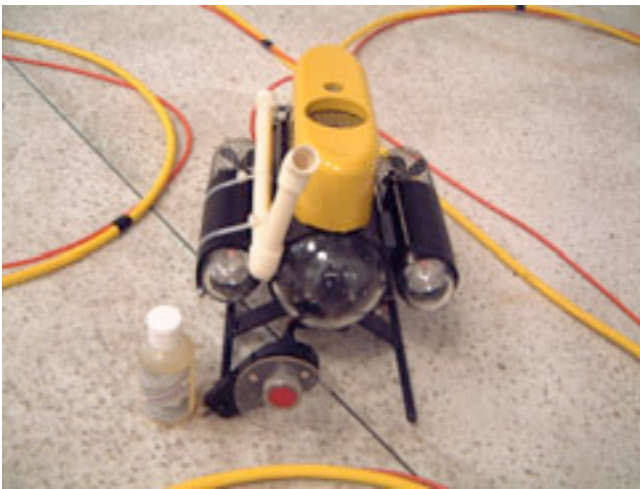
VideoRay with overhead sampling tray as well as Cygnus IV Multi-Echo Ultrasonic Thickness Gauge attached. (Photo by Bob Christ)
