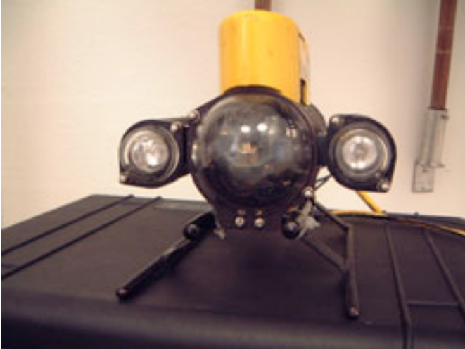
VideoRay with Dissolved Oxygen probe attached on the bottom of the starboard-side hull (Photo by Bob Christ)
