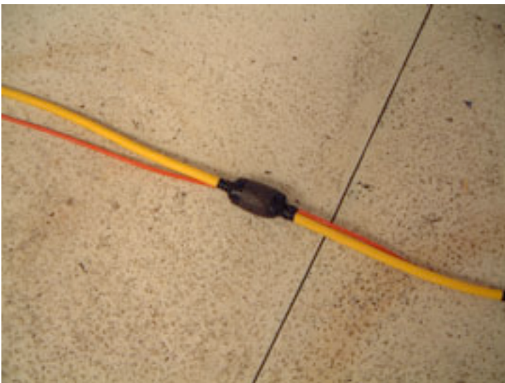
Tapered float on junction of instrument cable attachment to VideoRay tether (Photo by Bob Christ)
